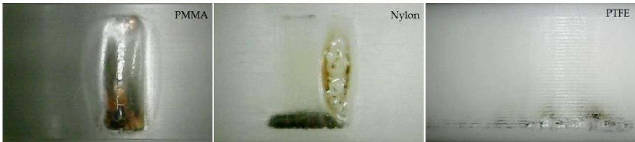
Figure 18. Surface damage of different materials under 50 Hz RMPs.
