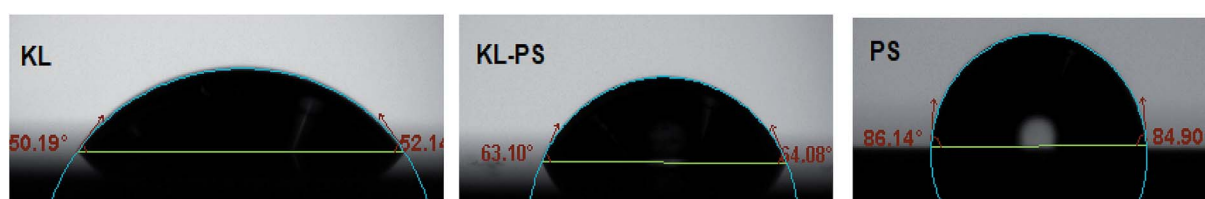
Fig. 3 Contact angle images of water droplet on KL, KL-PS and PS coated substrates.
