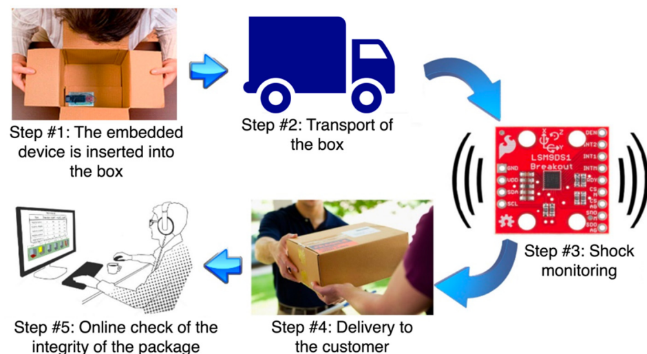
Figure 5. Stages of the shock monitoring system for the transport of goods.
