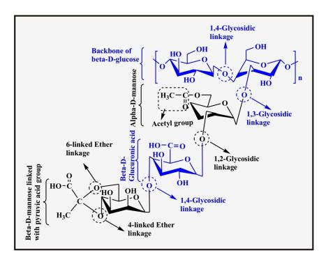
Figure 8. Chemical structure of Xanthan.
