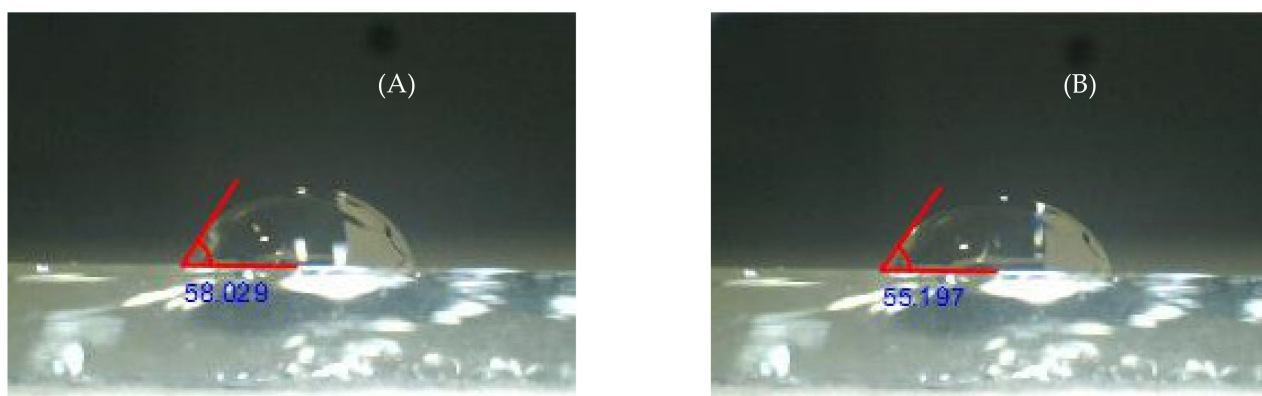
Figure 3. Contact angle of water droplet with 20 \mu L of volume on Ti/Ag/Ti/Ag film (A) t = 0 s and (B) t = 120 s.
