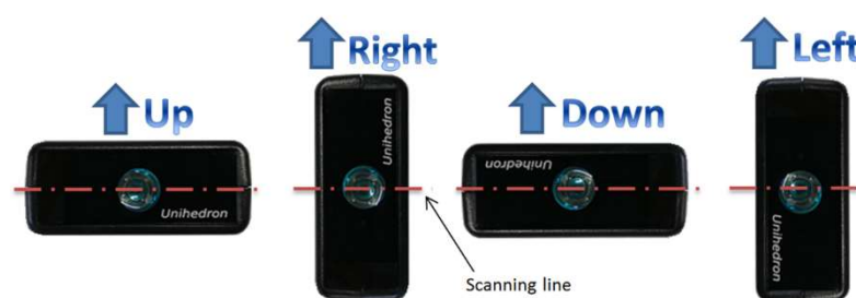
Figure 4. Overview of SQM unit orientation during measurements.
