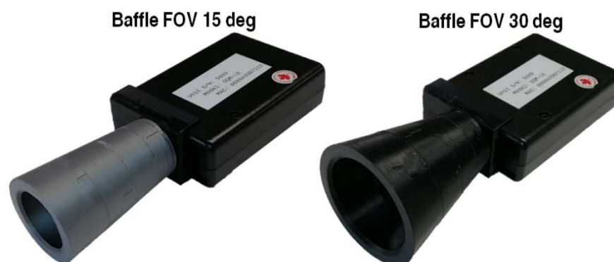
Figure 15. 15 deg baffle (left) and 30 deg baffle (right) integrated on SQM unit.
