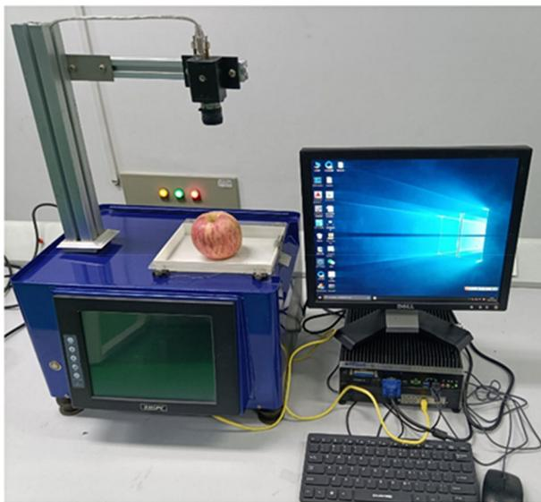
**Figure 13.** The online detection system for apple quality detection.
