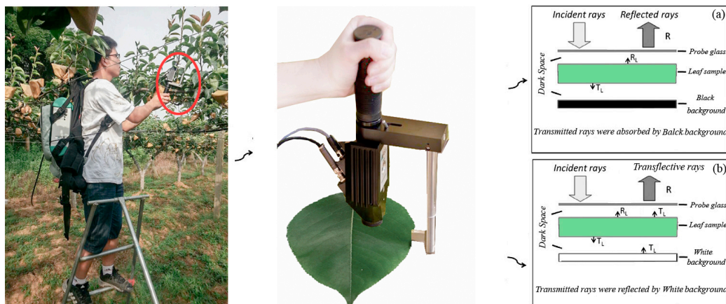
Figure 1. The schematic diagram of spectral acquisition by two methods. The reflectance measured with the black background (a); and the transfectance measured with the white background (b).
