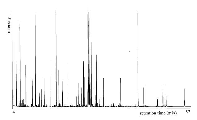
**Figure 1.** Polar phase of Solanum tuberosum leaves, analysed by GC/quadrupole MS (unpublished results). Inspection of peaks apparent in the base peak chromatogram results in some 150 distinct metabolites. Abundant peaks in the middle of the chromatogram are monosaccharides, followed by disaccharides (sucrose being the largest), and raffinose at the end of the chromatogram. Trimethylsilylated hydroxy- and amino acids are eluted in the first third of the profile
