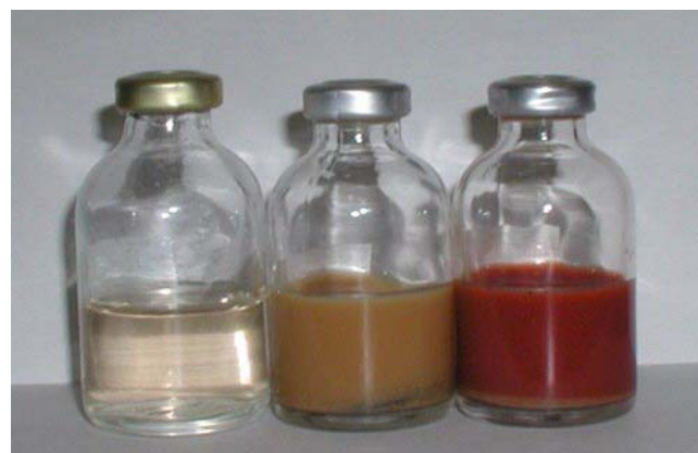
Figure 2 Color change resulting from the microbial reduction in soil of the respiratory dye XTT Bottle on the far left is a control of the oxidized dye in sterile water. The middle bottle shows lack of dye reduction by a sandy soil that was autoclaved. The bottle on the far right shows dye reduction (increase in orange color measurable at 465 nm) from a biologically active (contains living bacteria) sandy soil.
