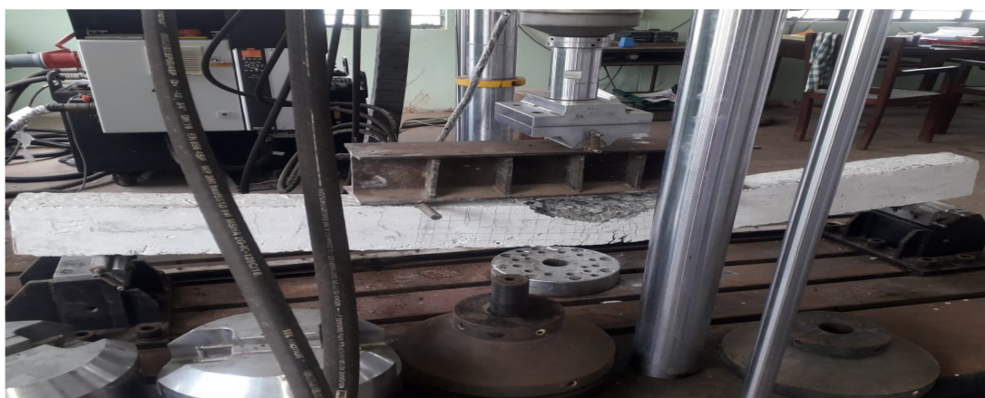
Figure 12. Failure pattern of RC beams.
