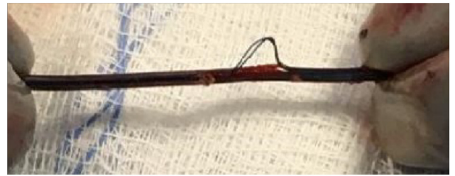
Figure 1 Externalized conductor in Riata lead postexplant.
