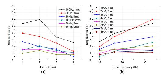
**Figure 9.** Response time of smooth muscle contraction under different stimulation parameters in rodent models. Response time is defined as the time difference between the end of stimulation and onset of smooth muscle contraction (a) Response time under different current intensities. (b) Response time under different stimulation frequencies. The electrical charge delivered into the bowl is within the safe limit of the electrode.
