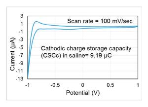
**Figure 7.** Measured cyclic voltammogram of the electrode array.
