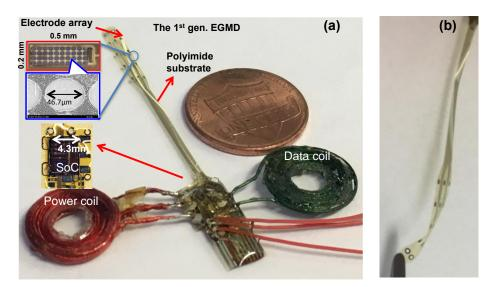
**Figure 5.** (a) Prototype of the miniaturized wireless EGMD. The high quality factor (Q) power coil is made by 100-strand litz wire (American Wire Gauge-48 (AWG-48)) with Q of >70 for high wireless power transfer efficiency and a data coil made of single wire (AWG-24) has low Q of ~5 to optimize data transmission bandwidth; (b) the flexible electrode array.
