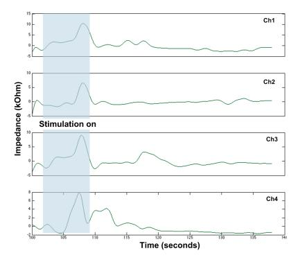
**Figure 10.** GI motility recording from the porcine model through impedance variation. Stimulus was applied to electrode #4, from t = 102 to t = 109. The measured results during this window are artifacts. Ch4 presents a contraction after t = 109.
