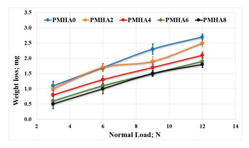
**Figure 10.** Wear of the PMMA/HA nanocomposites, with different HA weight ratios, rubbed against a PMMA surface under different normal loads.
