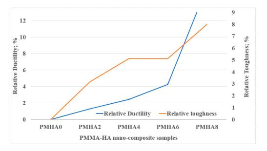
**Figure 5.** Relative toughness and ductility of the PMMA/HA nanocomposites with different HA weight ratios.
