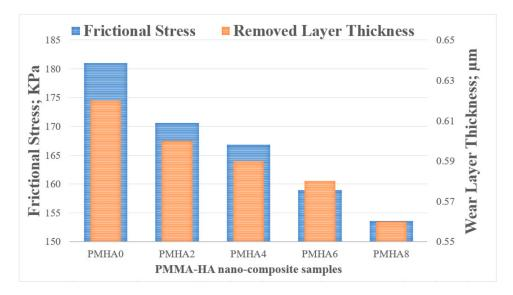
**Figure 14.** Frictional stress and wear layer thickness on the surface of the PMMA/HA nanocomposites, with different HA weight ratios.
