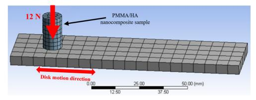
**Figure 11.** Finite element model of the friction test, including the poly(methyl methacrylate) (PMMA)/hydroxyapatite (HA) nanocomposite, rubbed against a stainless steel counterpart.
