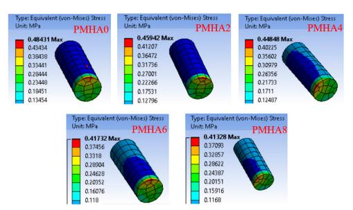
**Figure 12.** Equivalent stress distribution along the surface of the PMMA/HA nanocomposites, with different HA weight ratios.
