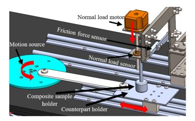
Figure 2. Reciprocating pin-on-disk tribometer.
