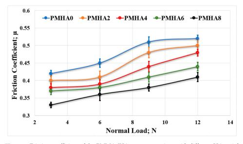
**Figure 8.** Friction coefficient of the PMMA/HA nanocomposites, with different HA weight ratios, rubbed against a PMMA surface under different normal loads.
