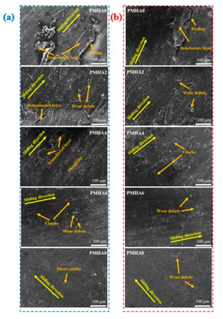
**Figure 15.** Scanning electron micrographs of the surface of the PMMA/HA nanocomposites, with different HA weight ratios, after being rubbed against (**a**) stainless steel or (**b**) a PMMA counterpart.
