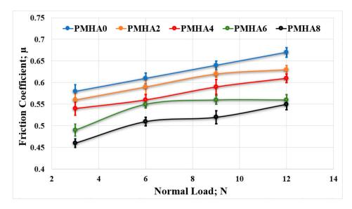
**Figure 7.** Friction coefficient of the PMMA/HA nanocomposites, with different HA weight ratios, rubbed against a stainless-steel surface under different normal loads.
