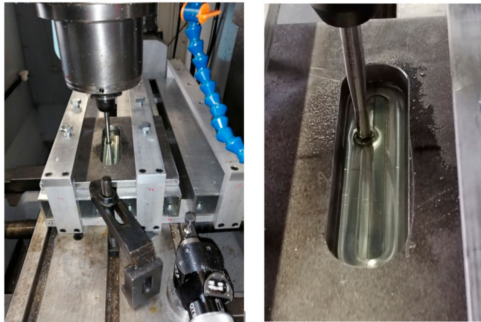
Figure 2. Device for incremental forming mounted in the table of a numerically controlled TM-1P vertical milling machine.
