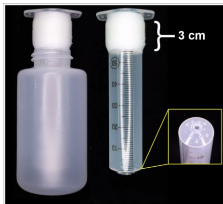
Figure 2. Apoplastic wash collection. Image showing 250 mL Nalgene bottles with 60 mL syringe modification for centrifuge apoplastic wash (cAW) isolation from Sorghum bicolor plants. The syringe is wrapped with parafilm (3 cm) to create a stopper between the tube and the syringe. The layer of parafilm is approximately 3 mm thick.
