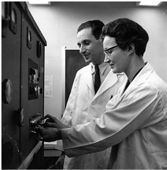
Figure 3. Drs. Michael and Kate Bárány operating a Beckman Model E ultracentrifuge to determine protein molecular weights. Photo provided by Dr. R. John Solaro.
