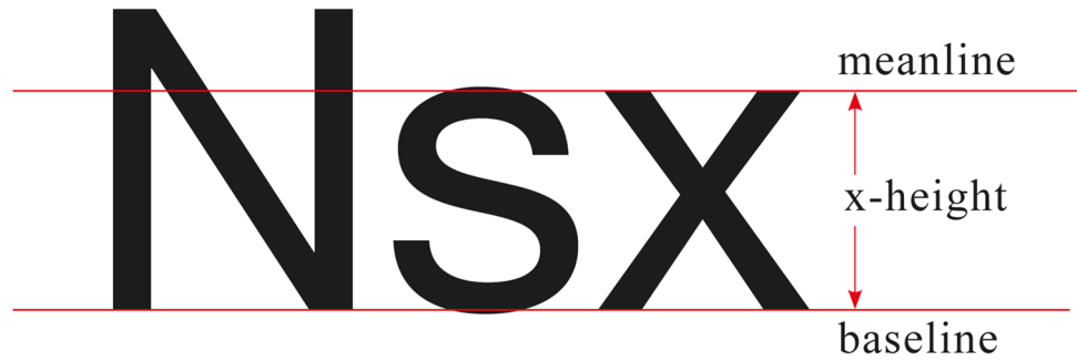
Fig. 2 Graphic representation explaining the x-height: The x-height (height of the lowercase “x”) represents the distance between the baseline and the mean line for a font. Lowercase letters with round parts such as the “s” exceed these heights (overshoot these lines)
