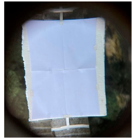
(b) the image detected by the telescope with pure Al mirrors
