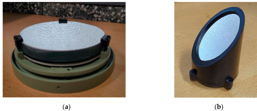
Figure 8. (a) Ag-enhanced primary mirror of the telescope, approximately 15 cm in diameter; (b) Ag-enhanced secondary mirror of the telescope, with a diameter of 5 cm.
