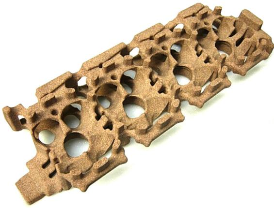
**Figure 1.** Water jacket core used during the manufacturing of cylinder heads.
