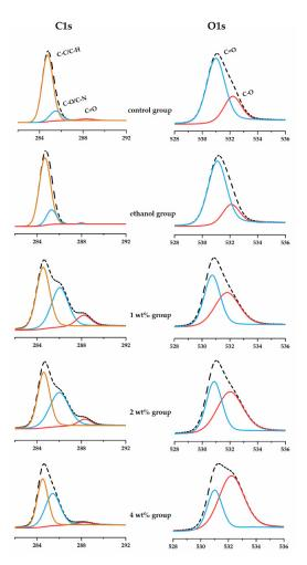
**Figure 5.** XPS high-resolution C1s (left column) and O1s (right column) spectra of dentin treated by irrigants.
