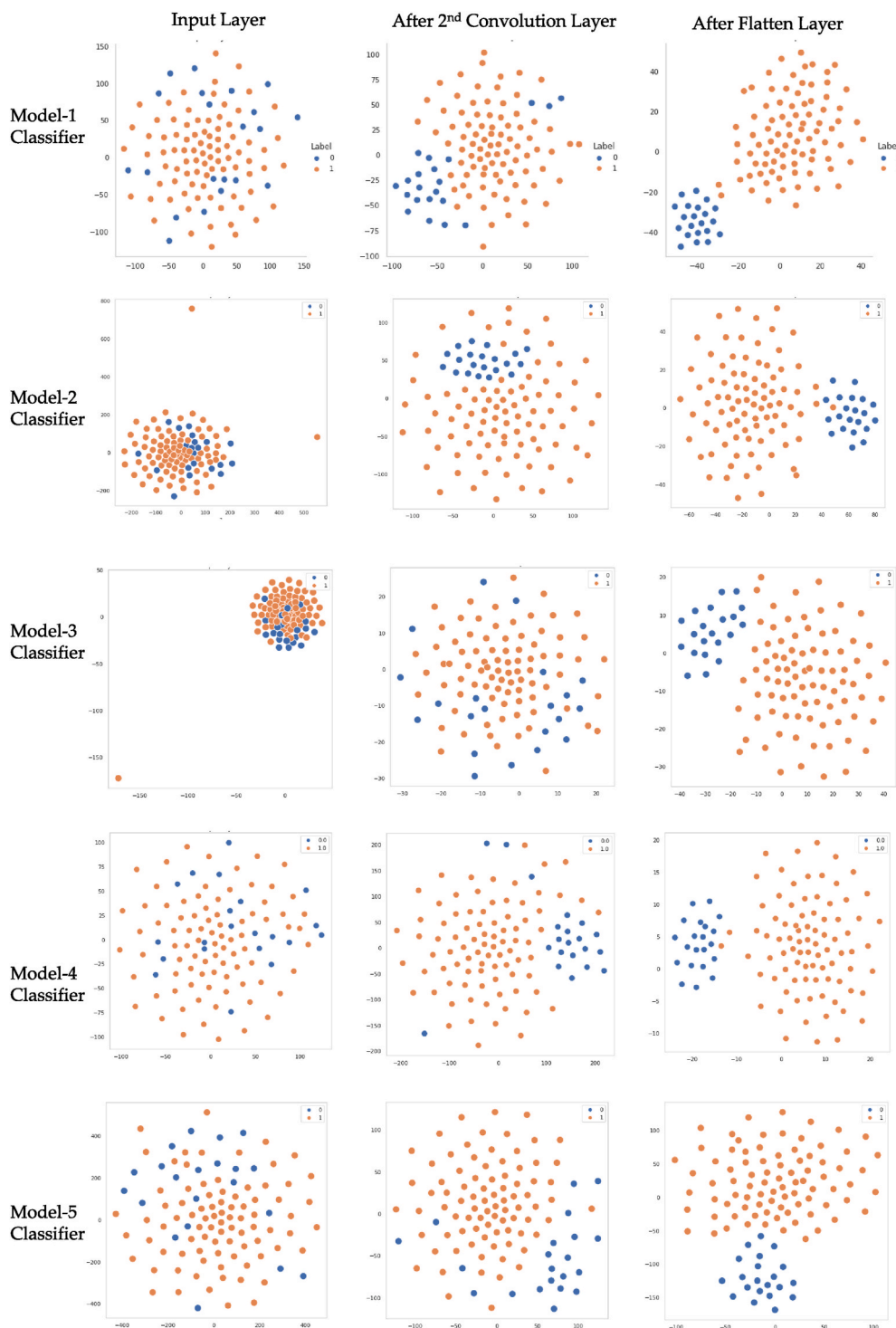
Fig. 3. t-SNE plots of ECG data being separated layer after layer when features are learnt gradually by the ECG-iCOVIDNet model.
