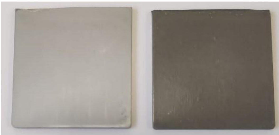
Figure 5. (Left): Plaque of amorphous PET with Al nano platelets is silvery. (Right): Plaque of amorphous PET with nodular Al particles is dark grey. The appearance is directly related to the particle shape.
