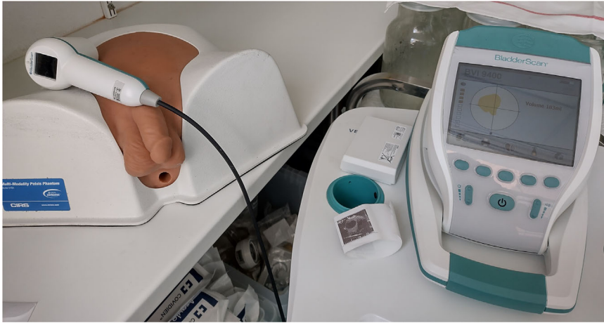
FIGURE 1 BladderScan BVI 9400 and CIRS multimodality 048A phantom. The screen displays if the bladder is correctly centered
