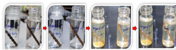
Fig. 38 Effect in degassed and distilled water on rusting with Fe scrap.
