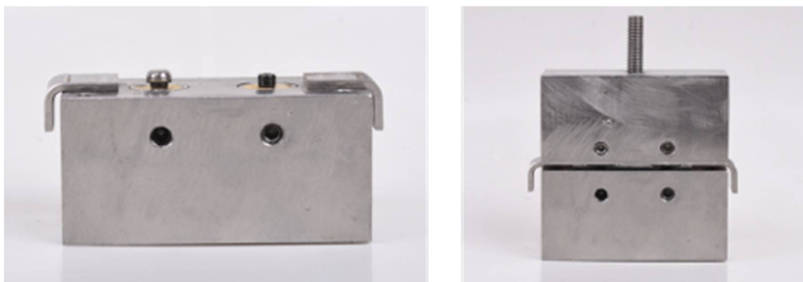
Figure 2. A metal spacer used to provide space between the upper and lower specimens.
