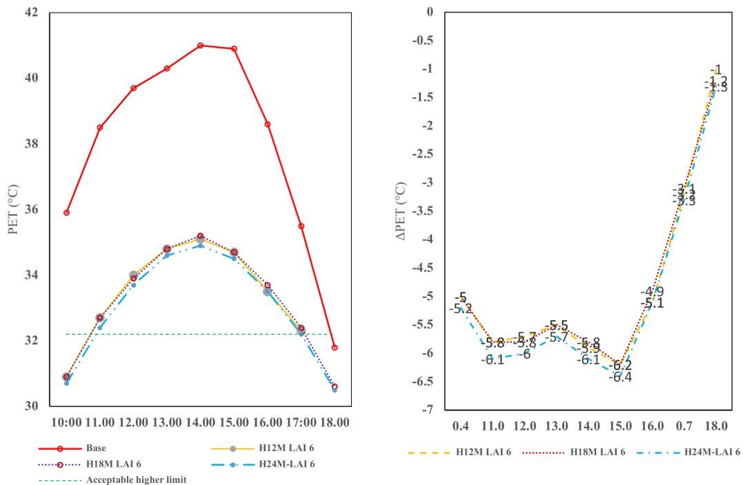
**Fig. 11.** The influence of combination of building height and vegetation on outdoor thermal comfort in informal settlement. The dotted green line (Fig. 11a indicates upper comfort limit. (For interpretation of the references to colour in this figure legend, the reader is referred to the Web version of this article.)
