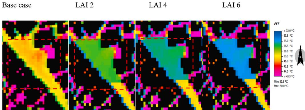
Fig. 7. The influence of addition of trees on the outdoor thermal comfort at pedestrian height (1 m) showing reduction of PET for different LAI.
