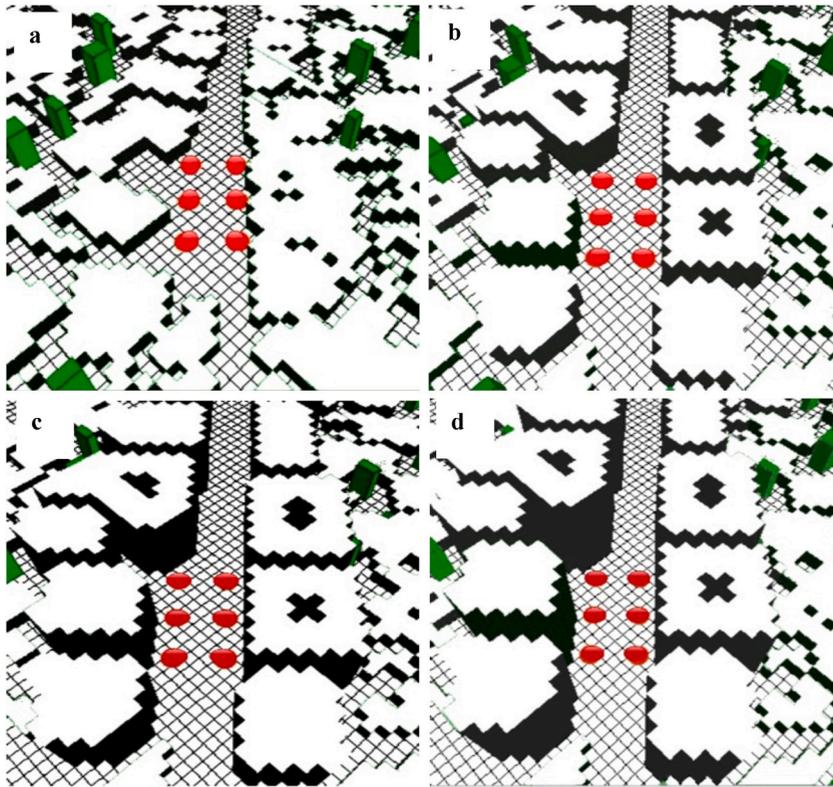
**Fig. 2.** A 3d representation of (a) existing 4 m height model (b) 12 m height model (c) 18 m height model, and (d) 24 m height model for Tandale informal urban fabric area. The red dots show the positions of the receptors. (For interpretation of the references to colour in this figure legend, the reader is referred to the Web version of this article.)
