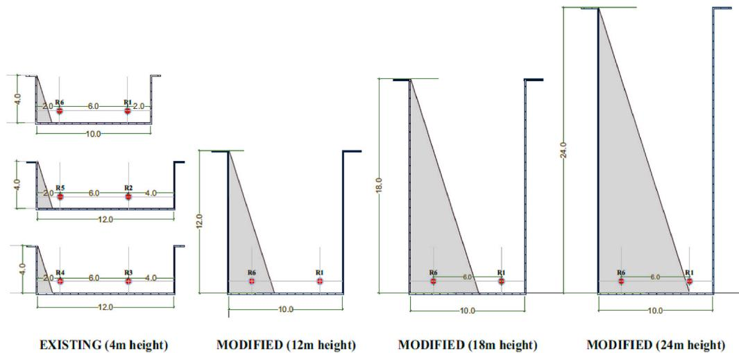
**Fig. 3.** Schematic cross-sections of urban canyon scenarios which involves changes of height from existing low-rise (4 m) to 12 m, 18 m, and 24 m. Red dots indicate position of receptors where microclimate variables were analysed. (For interpretation of the references to colour in this figure legend, the reader is referred to the Web version of this article.)
