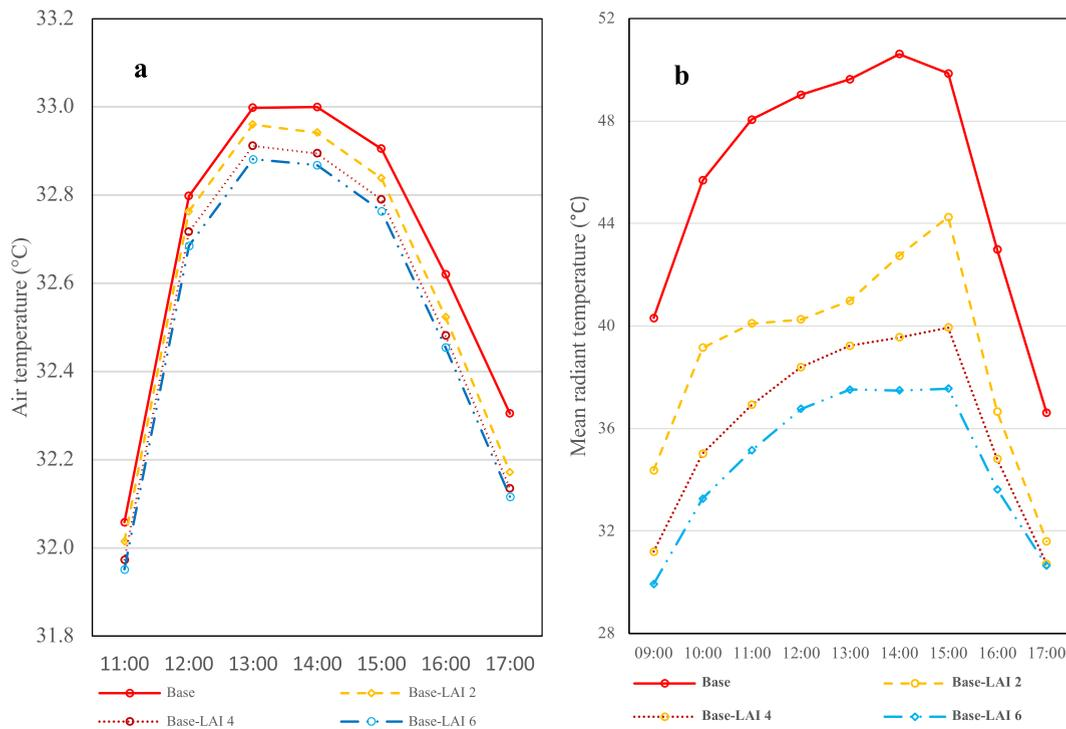
Fig. 4. The influence of addition of trees with different LAI on (a) air temperature and (b) mean radiant temperature in the informal urban fabric at pedestrian height (1 m).
