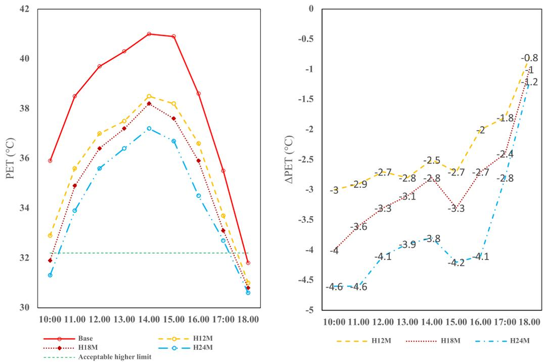
**Fig. 9.** The influence of increase in building height on outdoor thermal comfort at pedestrian height (1 m) in the informal settlement. The green and dashed horizontal line (Fig. 11a) represents upper comfort limit. (For interpretation of the references to colour in this figure legend, the reader is referred to the Web version of this article.)
