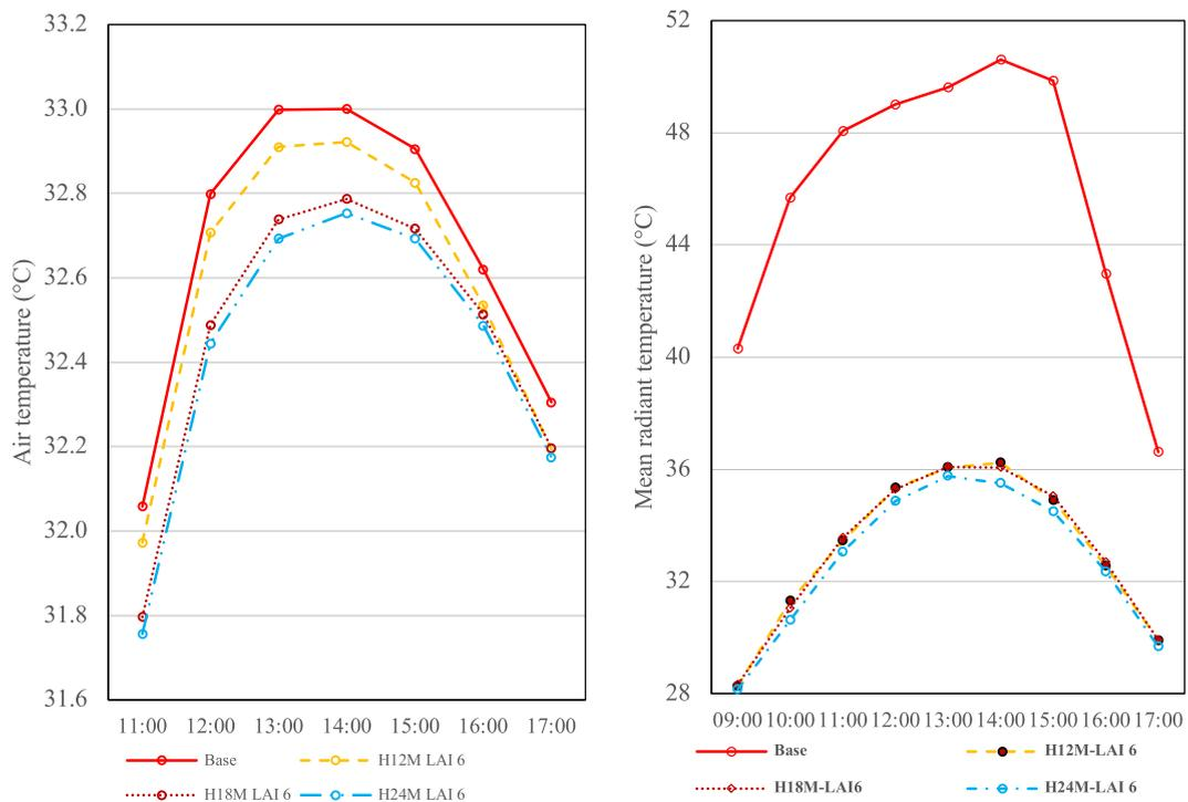
**Fig. 10.** The influence of combination of building height and vegetation on (a) air temperature and (b) mean radiant temperature at pedestrian height (1 m) in the studied informal urban fabric.
