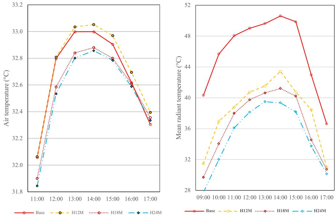
**Fig. 8.** The influence of an increase in building height on air temperature (a) and mean radiant temperature (b) within the informal urban fabric.
