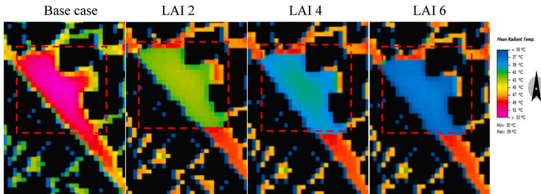
Fig. 5. The influence of addition of trees with different LAI values on mean radiant temperature in the informal urban fabric at pedestrian height (1 m) at 2:00pm.
