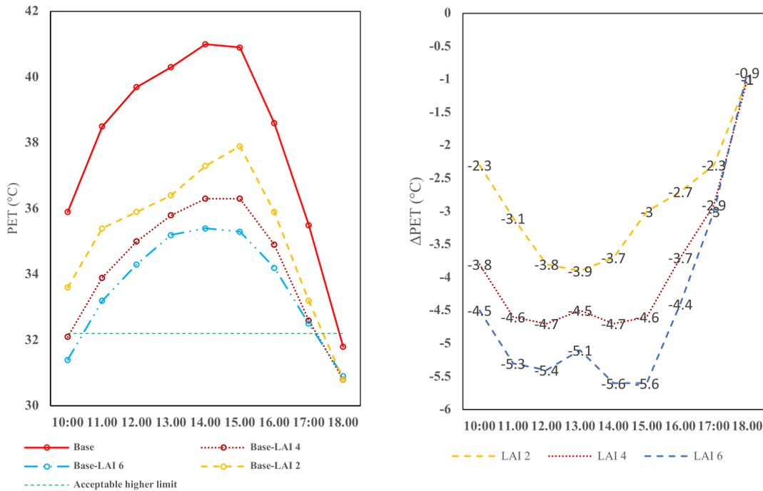
Fig. 6. The influence of addition of vegetation on the outdoor thermal comfort at pedestrian height (1 m) (a) and reduction of PET for different LAI values (b).
