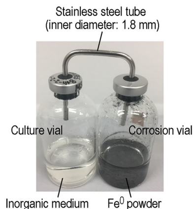
Figure 2. The iron corrosion-assisted H 2 -supplying (iCH) system. The vial on the left is for culture of microorganisms and that on the right is for the iron corrosion (i.e., H 2 production) reaction. The gas phases of the two vials are connected by a stainless steel tube to allow diffusion of H 2 produced in the corrosion vial.
