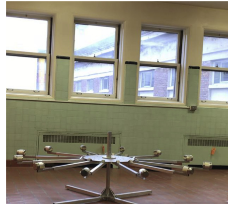
Figure 1. Scent wheel used for canine team inter-rater reliability testing. The scent wheel has 12 arms that can be set at different distances and the carousel can be set to various heights. The wheel can be rotated. Canisters containing the odours of interest are used once before being washed in an industrial washer.
