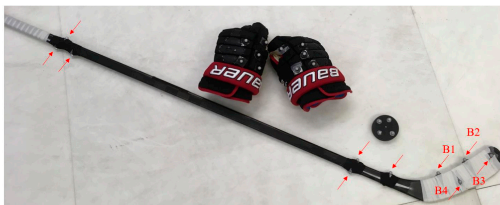
Figure 2. Reflective marker placement on gloves, stick, and puck for tracking by the Vicon system. B1–4 indicate markers used to define the movement of the stick blade during the shooting trials.
