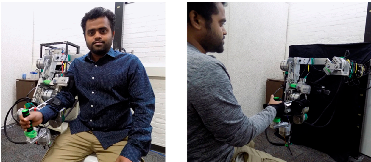
Figure 17. On the left , the subject is wearing u-Rob as an exoskeleton-type setup for joint-based exercises, whereas on the right , the subject is wearing u-Rob as an end-effector-type setup for end-point exercises.
