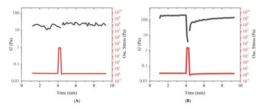
Figure 3. Recovery behaviour of PCL (A) and PCL-CCG 0.5 (B) under stress.
