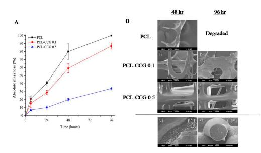
**Figure 8.** Mass loss study of MEW PCL scaffolds via enzymatic degradation (**A**); SEM images of scaffolds after enzymatic degradation (**B**) at 48 h (Bi–iii) and 96 h (Biv,v). High magnification cross-sectional images of PCL (Bvi) and PCL-CCG 0.5 (Bvii).
