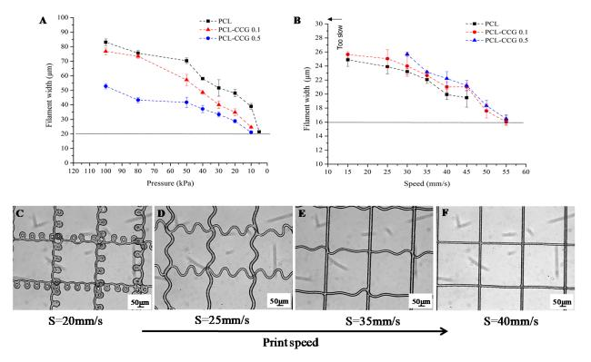
**Figure 5.** Filament width of MEW PCL against (**A**) pressure and (**B**) speed. As printing speed increases (**C**–**F**), the coiling of fibres reduced until a critical speed of 40 mm/s is reached.
