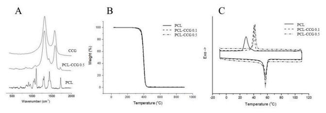
Figure 4. Raman spectra (A), TGA (B) and DSC (C) curves of PCL and PCL-CCG composites.
