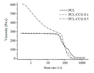
Figure 2. The apparent viscosity value of the PCL and PCL composites as a function of shear rate.
