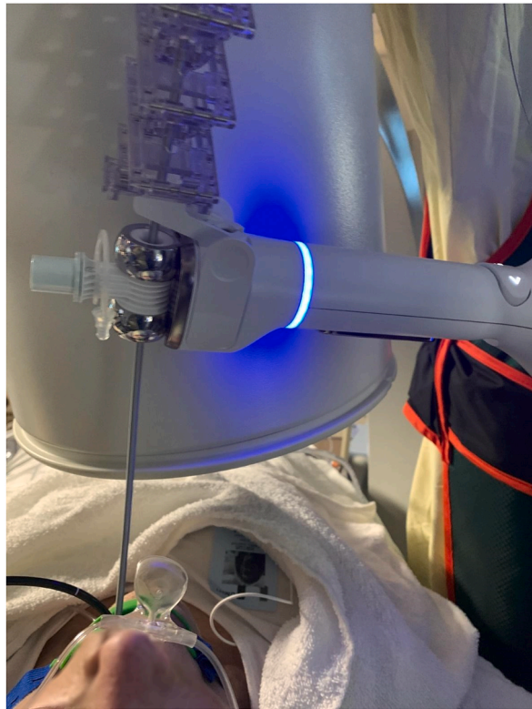
Fig. 1. ION robotic bronchoscopy setup: silver magnetic swivel adapter connected to robotic arm and robotic catheter going through the mouth.
