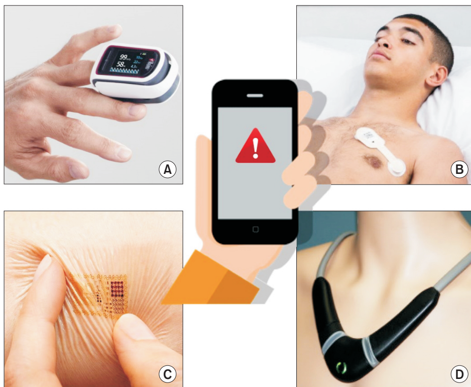
Fig. 6. Example of mobile monitoring systems for ambulatory patients and/or home monitoring. A = pulse oximeter from Masimo.com, B = adhesive patch from Isansys.com, C = electronic tattoo from mc10inc.com, D = Necklace from Tosense.com. The information is transmitted to a mobile display (e.g. a smartphone) so that healthcare professionals and/or patients are informed early in case of clinical deterioration.
