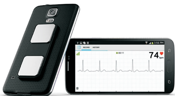
Fig. 7. Example of smartphone case for electrocardiography (ECG) recording. This case includes 2 electrodes. Putting fingers on the electrodes enables the recording of a single lead ECG that can be recorded and shared with healthcare professionals. From Alivecor.com.
