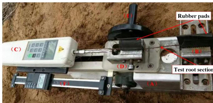
**Figure 3.** HG 100 digital display type push-pull meter and self-made portable test instrument.
