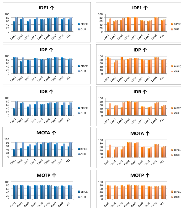
Figure 11. Comparison between the benchmark and ours. The IDF1, IDP, IDR, MOTA and MOTP arranged from top to bottom, and the bar graphs on the left are the results of test-easy set, the rights are the results of test-hard set.
