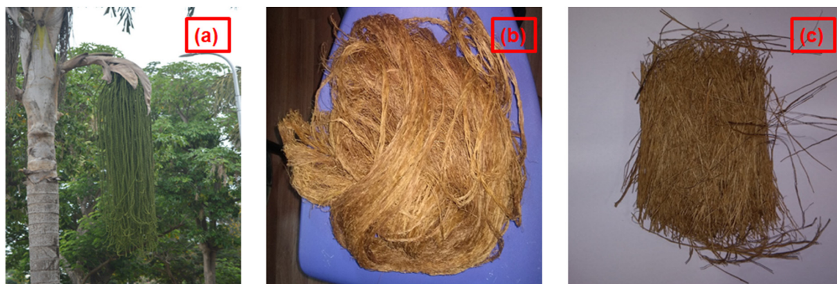
Fig. 1. Fish tail palm fibre processing (a) fish tail palm tree, (b) extracted fish tail palm fibre, and (c) chopped fish tail palm fibre.
