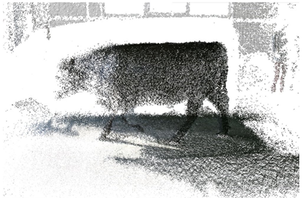
Figure 2. 3-D point cloud model of the cattle using the proposed system for 3-D reconstruction.
