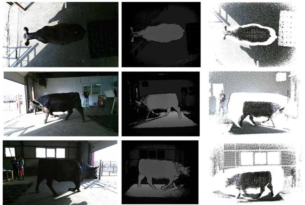
Figure 1. RGB images, depth maps, and point clouds of the cattle captured with three Kinect cameras.
