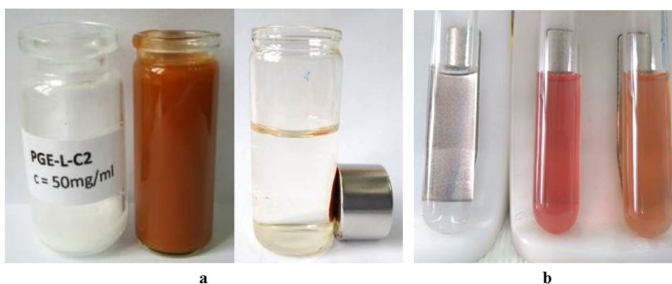
Figure 5. Light photographs documenting (a) the magnetic separation of Mag-P(CMMA-EDMA) particles (from left to right: P(CMMA-EDMA) and Mag-P(CMMA-EDMA) particles twice) and (b) the peroxidase-like activity of the blank, Mag-P(CMMA-EDMA), and Mag-P(CMMA-EDMA)-Th particles (from left to right).
