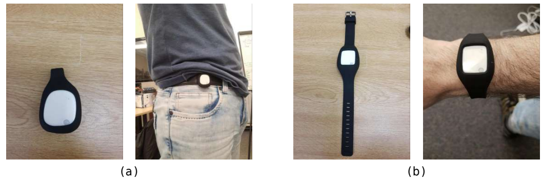
Figure 2. Inertial sensors attached to (a) a waist clip; and (b) a wrist band.
