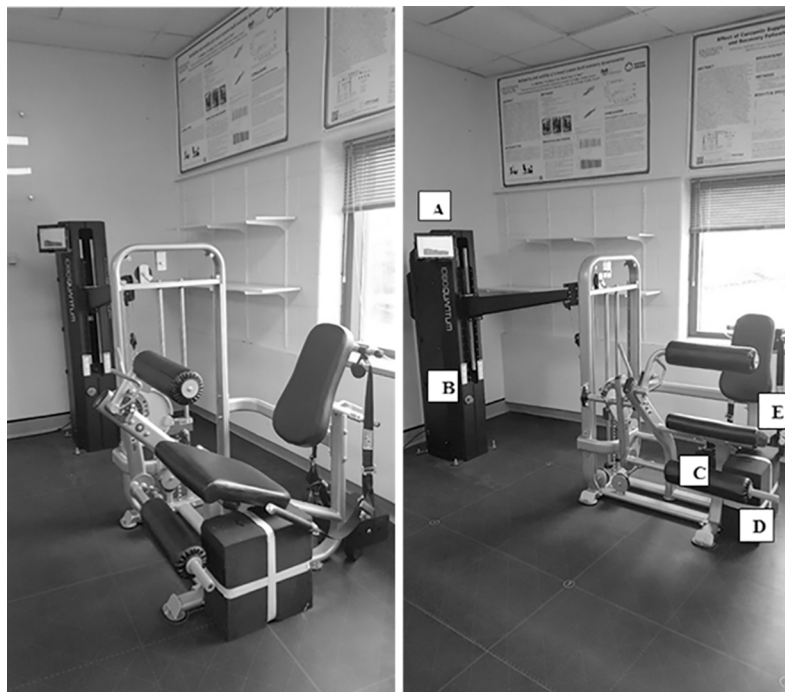
Fig 1. Configuration of the 1080 Quantum attached to Model A leg extension. The power outputs (W) would be presented on the A. tablet, calculated from the B. 1080 Quantum. The participant would sit in the leg extension machine and kick the C. movement arm outwards to complete the leg extension. The D. range of motion apparatus was in place to suspend the extension, bringing the participant's leg back to the neutral position to be prepared for subsequent extensions. Finally, the participant was secured with a E. harness.
