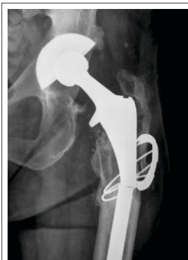
Figure 3: Case 2: Radiograph showing fracture through an Echelon™ stem just distal to the extended trochanteric osteotomy site
