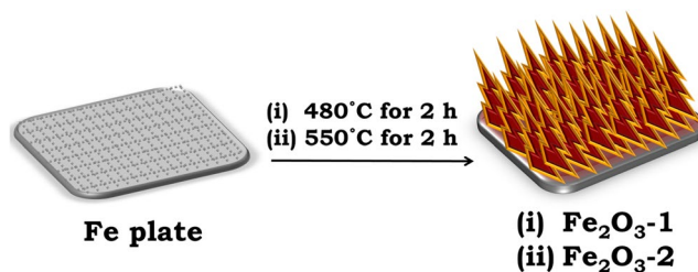
Figure 1. Schematic diagram for fabrication of \text{Fe}_2\text{O}_3 nanowires.
