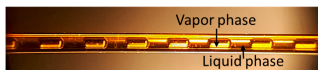
Figure 3. Picture of the segmented flow in the glass capillary.
