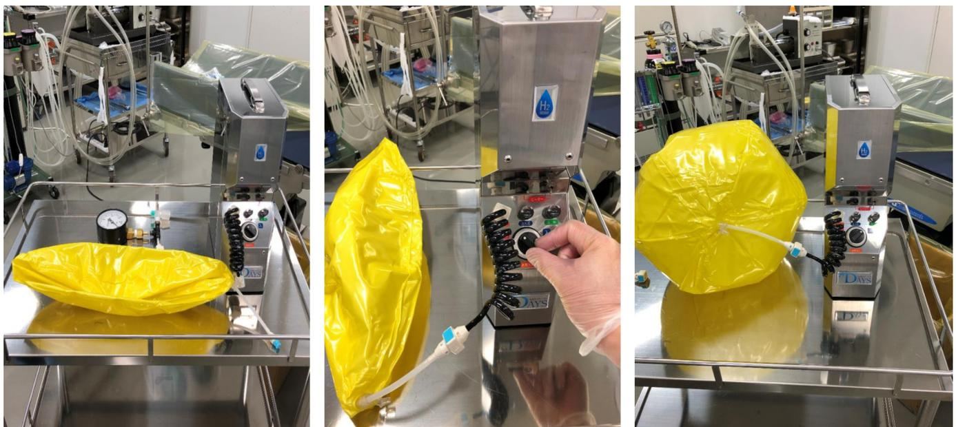
**Fig 1. Beach ball being filled with 100% H<sub>2</sub>.** The ball is expanding with H<sub>2</sub> released from a hydrogen-absorbing alloy in an H<sub>2</sub> filling device.
