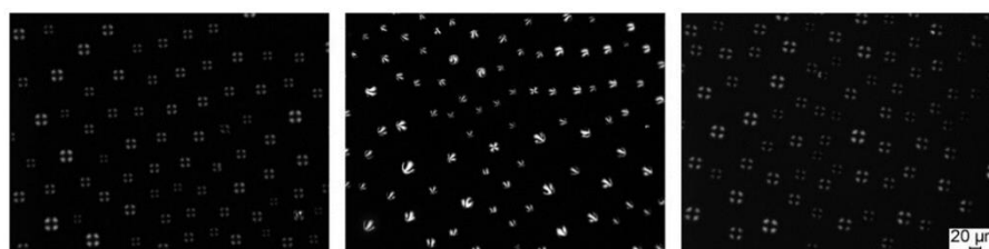
Figure 3. Polarized light microscopy images of surface-anchored LC droplet patterns in a different solution. Reprinted with permission from ref. [73]. Copyright 2014 John Wiley and Sons. The scale bar is 20 \mu\text{m} .
