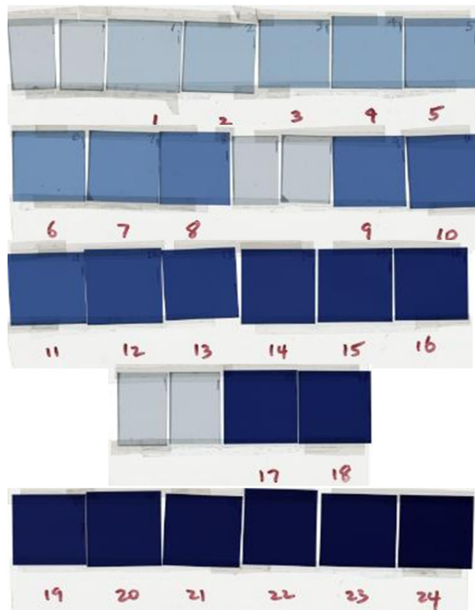
Figure 2 Scanned images of the calibration EBT films obtained in this study. The doses to the calibration films ranged from 20 (film #1) to 5000 cGy (film #24). The films without number label were background films kept in this set.
