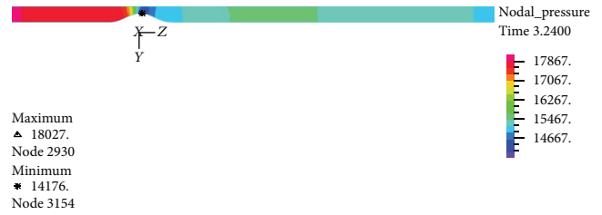
FIGURE 25: Pressure distribution at maximum flow rate T_2 , FSI-Turb.
