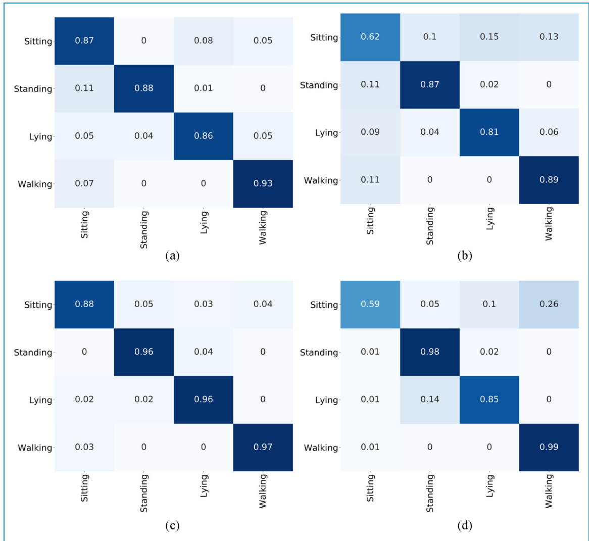
Figure 10. Confusion matrix for different models of ACC + ECG signals on the dataset of the pneumoconiosis patient group: (a) CNN; (b) LSTM; (c) CNN-LSTM; (d) GRU.
