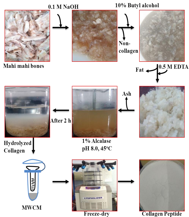
Scheme 1. Schematic illustration of extraction steps involved in isolation of collagen peptide from Mahi mahi bone. MWCM: molecular weight cut-off membrane.
